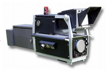
The camera is fully transistorised, except for the HV rectifiers and it uses the 4.5" I.O. tube with the latest Elcon target material, Elcon stands for "electronic conducting" and it removed the stickiness problem of earlier tubes.
