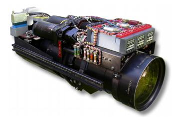
A choice of zoom lenses from different manufacturers, with different focal lengths and ranges could be fitted to the common lens mount.
