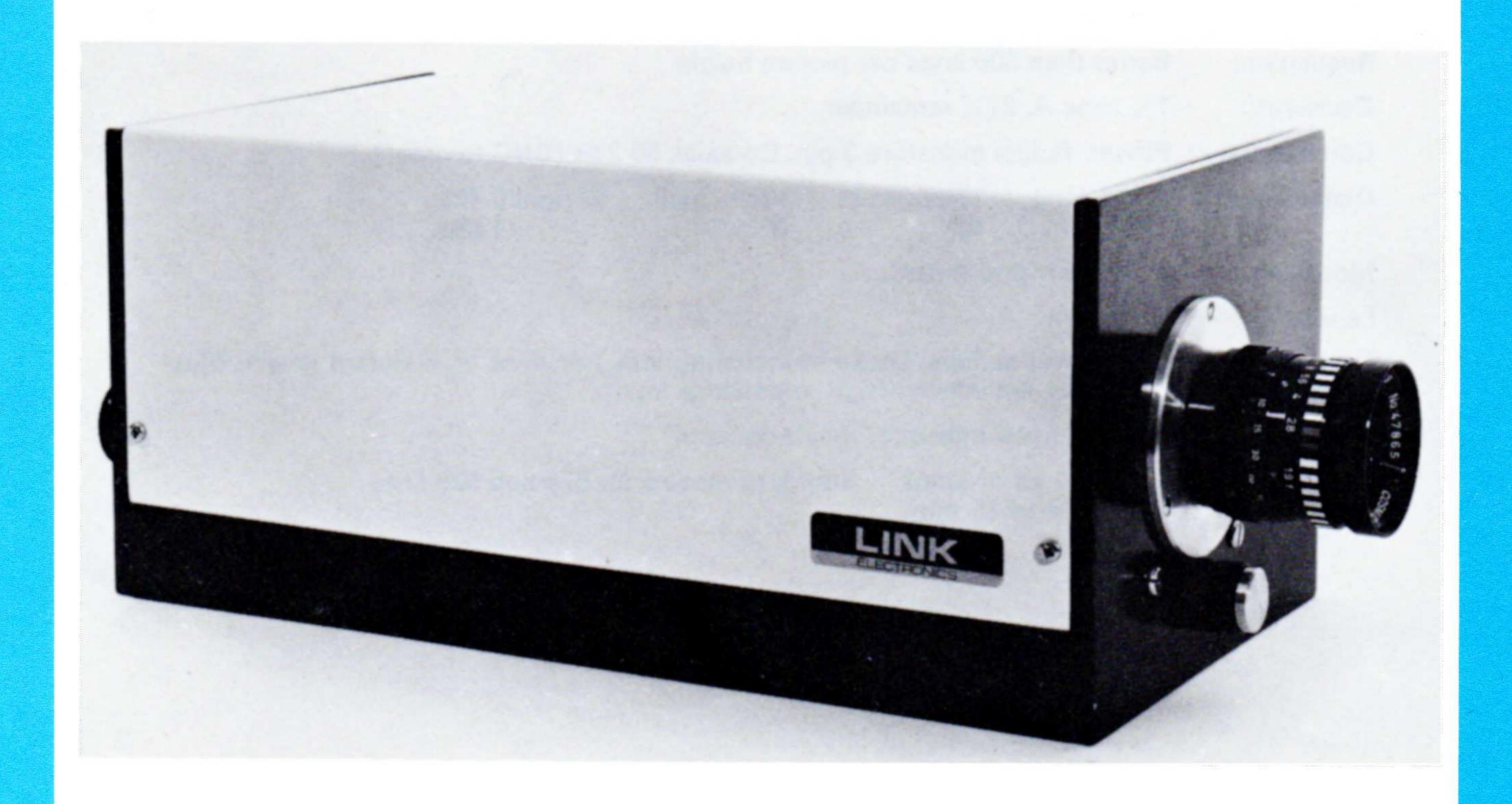
A completely solid state television camera for closed circuit and educational television using the separate mesh type of Vidicon pick-up tube. The camera is self-contained and has no operating controls apart from optical focus and on/off switch. Automatic sensitivity control maintains a sensibly constant output over a wide range of light levels. Two versions of the camera give either random interlace with external locking facility (101) or a built in 2:1 mains locked pulse generator (106).
