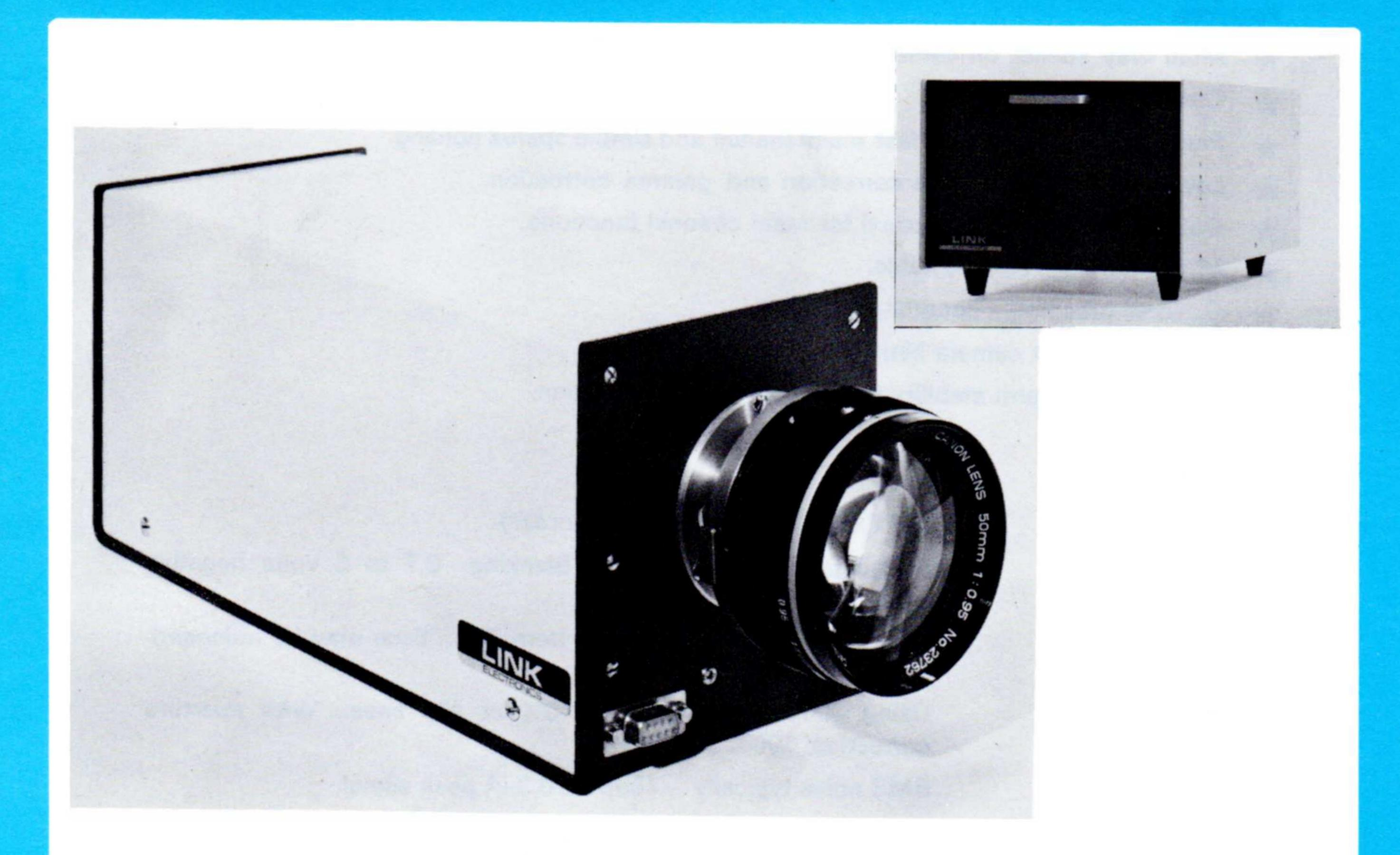
The type 104 television camera is designed for use as a caption or telecine camera, or as a non-viewfinder camera for use in remote unattended studios. It is designed to full broadcast standards and is the same basic channel as used in the type 103 studio/O.B. camera. This simplifies spares stocking and maintenance where the 103 and 104 cameras are used together.
