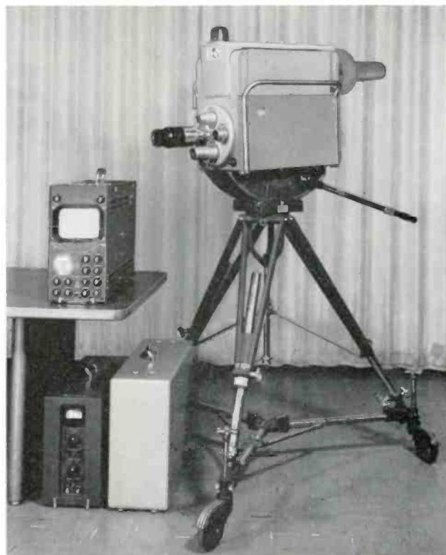
TK-14 Field Camera Chain showing Field Camera Control on table, TY-31A Field Power Supply and Field Case containing Focus Current Regulator and Electro-magnetic Orbiter Generator beside camera and viewfinder mounted on field tripod and dolly.
