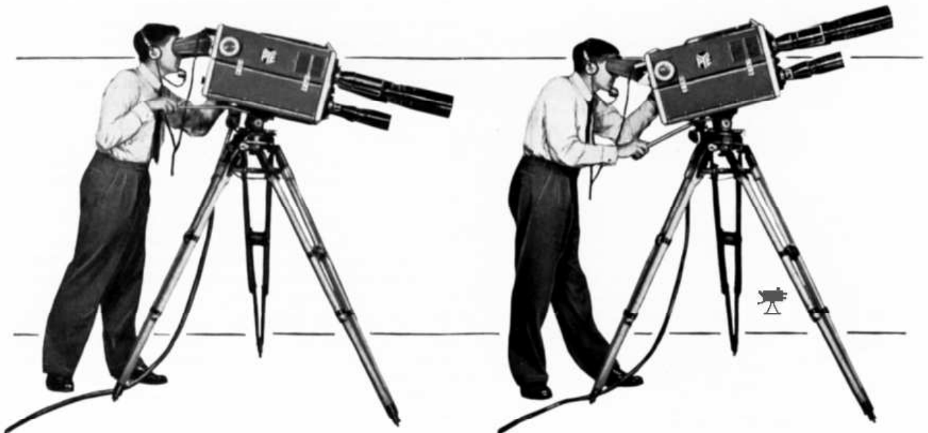
Two positions of viewfinder hood showing operating advantage.
