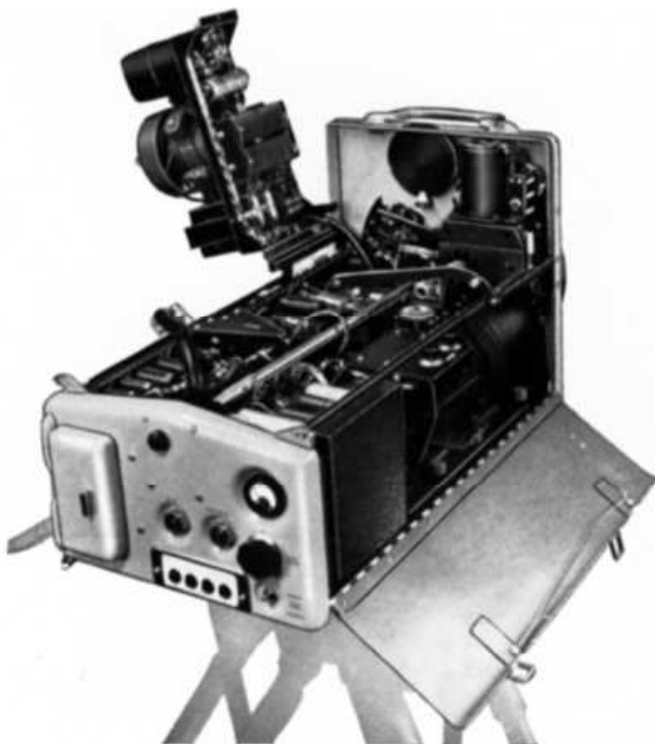
Viewfinder unit removed. Servo unit raised for servicing.
