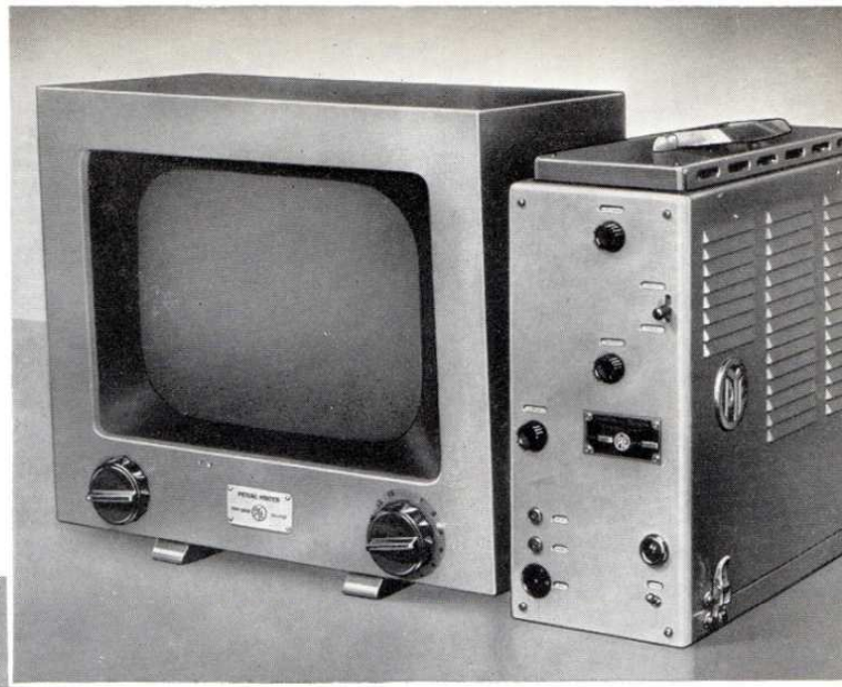
Camera Control Unit Type 2317, and Monitor Type 2812 employing a 14 inch rectangular picture tube.
