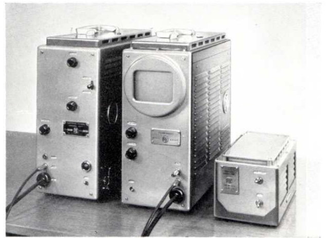
Camera Control Unit, 5 inch XXXXXXXXXX Monitor Type 2737, and Dual Lens Turret Control Unit.
