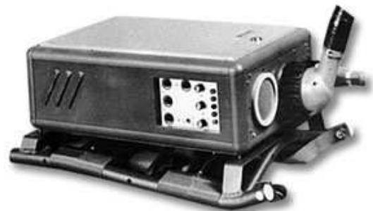
The LDK13 electronics backpack & frame
