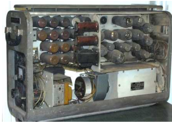
Figure 4. The PSU before restoration started
