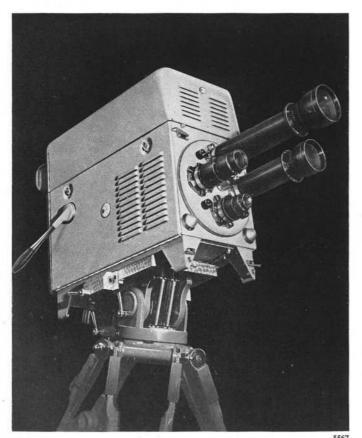
A VARIETY of techniques are at present employed in the design of television cameras. The Marconi Company has aimed to produce a small, compact unit, suitable for both studio and outdoor operation and giving the finest overall performance while, at the same time, being suitable for operation on all present-day transmission systems. This has been achieved by the use of the image orthicon tube.
