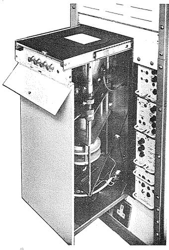
The tube carriage drawn forward for tube removal. plate and base-end clamp support the tube. No mechanical adjustments are necessary as tube alignment, with normal scans ON, is entirely, electrical using the four controlknobs shown at the front of the tube carriage. An inter-lock arrangement breaks the e.h.t. supply when the tube carriage is withdrawn.
