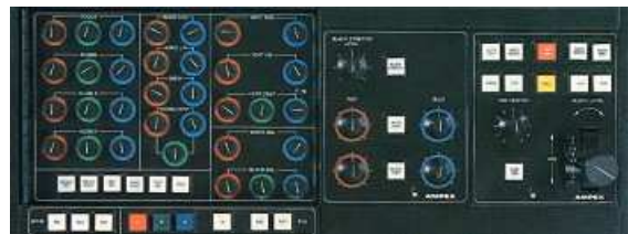
Master Control Panel for BCC 10
